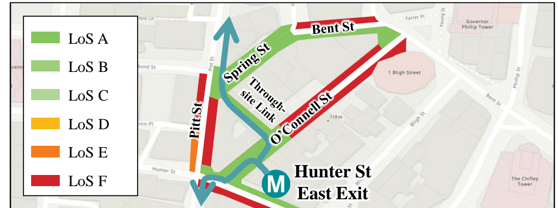
Figure 44: Future conditions combined with through-site link movements, Hunter Street movements and City North Public Domain Plan proposed changes
